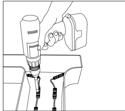
5. **Fasteners:** If desired, modules can be secured with #6 (3.5 mm) pan head sheet metal screws or 1/8 in (3 mm) aluminum rivets.
