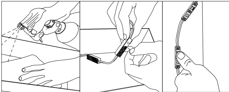
4. **Peel and stick:** Clean inside sign with rubbing alcohol and allow to dry. Using predetermined layout and LED placement from Step 3, remove tape backing and stick modules into place. Ensure modules are firmly attached. **CAUTION:** When handling modules, avoid pressing down directly on top of LEDs.
