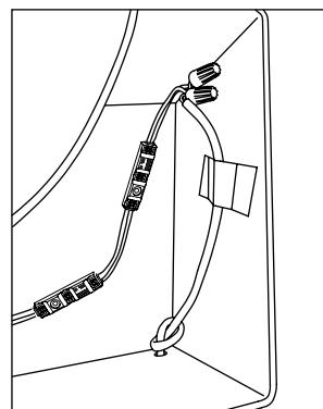
8. **Connect power supply to first module on string:** See Power Supply Install Guide for more information regarding power supply installation.
