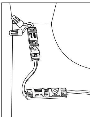
7. **Cap all unused wires:** The strand of modules should not be looped to create a closed circuit.
