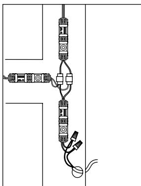
6. **Connections:** Modules may be connected in series or parallel.
